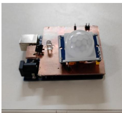
Figure 9 – Prototype of the PCB attached to the Arduino UNO R3
