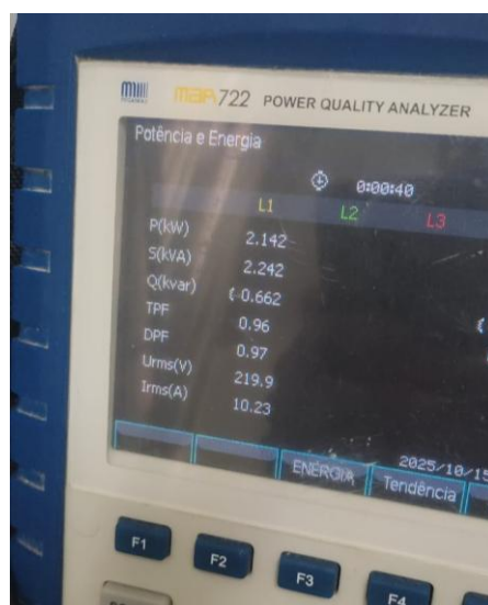
Figure 11 – Field data collection using an energy analyzer
